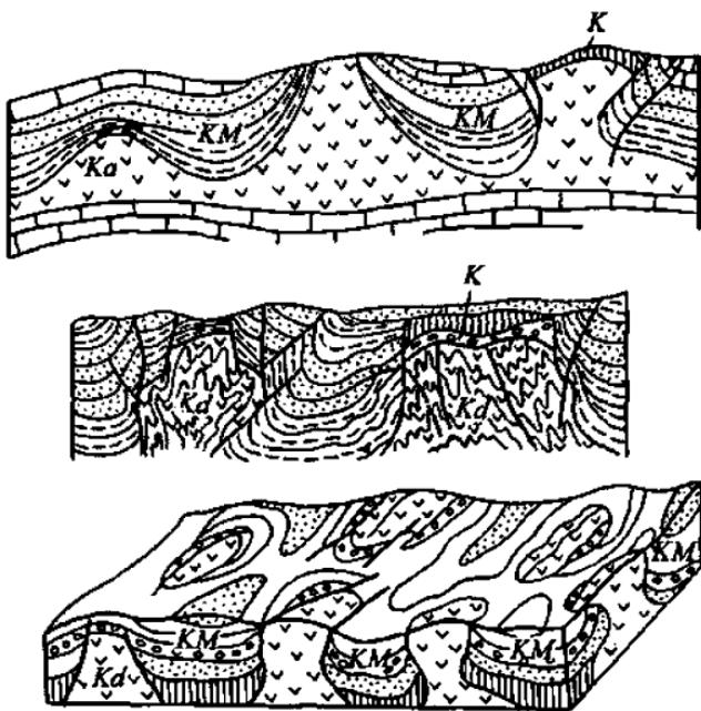
60-rasm. Diapirli burmalar. KM-kompensatsion mulda, Kd-criptodiapir, K-kelrok (V.N.Pavlinov bo'yicha).
