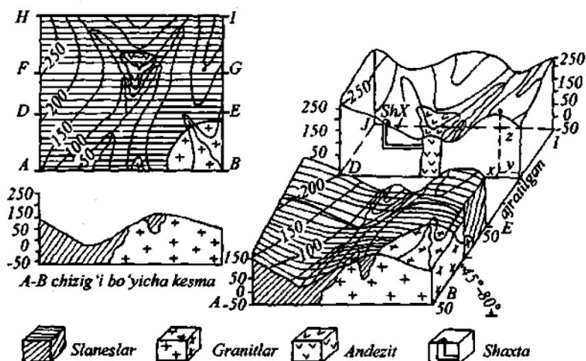
130-rasm. Parallel kesmalar yordamida blok-diagramma tuzish.
