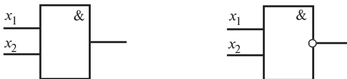
4.5-rasm. y = x_1 \cdot x_2 = (x_1 \wedge x_2) . 4.6-rasm. y = \overline{x_1 \cdot x_2} = \overline{(x_1 \wedge x_2)} .
