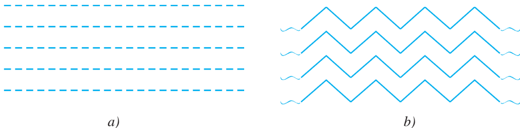
33-rasm. Parallel va zig-zak baxyaqator tikish: a – qo'sh chok; b – ichki chok.
