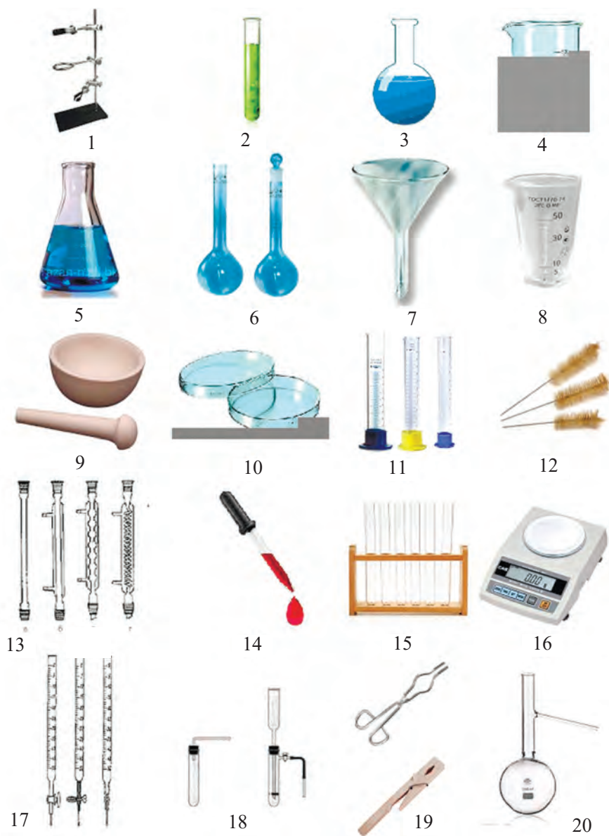
4-nji surat. 1–uniwersal ştatiw; 2–probirka; 3–düýbi togalak kolba; 4–ölçeg stakany; 5–konuşekilli kolba; 6–ölçeg kolbalary; 7–keramiki woronkalar; 8–menzurka; 9–keramiki soky daşy; 10–Petri gaby; 11–ölçeg silindrleri; 12–probirka arassalaýjy; 13–sowadyjy; 14–pipetkalar; 15–probirka goýguç; 16–elektron terezi; 17–býuret kalar; 18–gaz alyjy gural; 19–gysgyçlar; 20–Výurs kolbasy.
