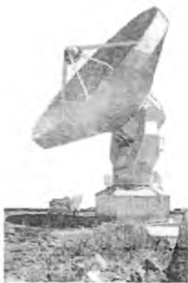
62-rasm. Parabolik antennali radioteleskop
